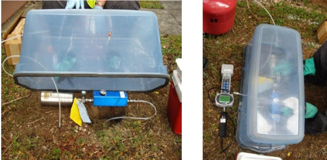
Figure 12 Covering the entire sampling system & probe with a shroud.
